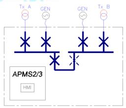
The APMS controller has been developed to manage split busbar LV power installations with circuit breaker and cable redundancy but can also be used at higher voltages. The most common model is the APMS2/5 for a "circular" system with two main busbars, three sources of supply available to each, including a bus-tie or buscoupler.
